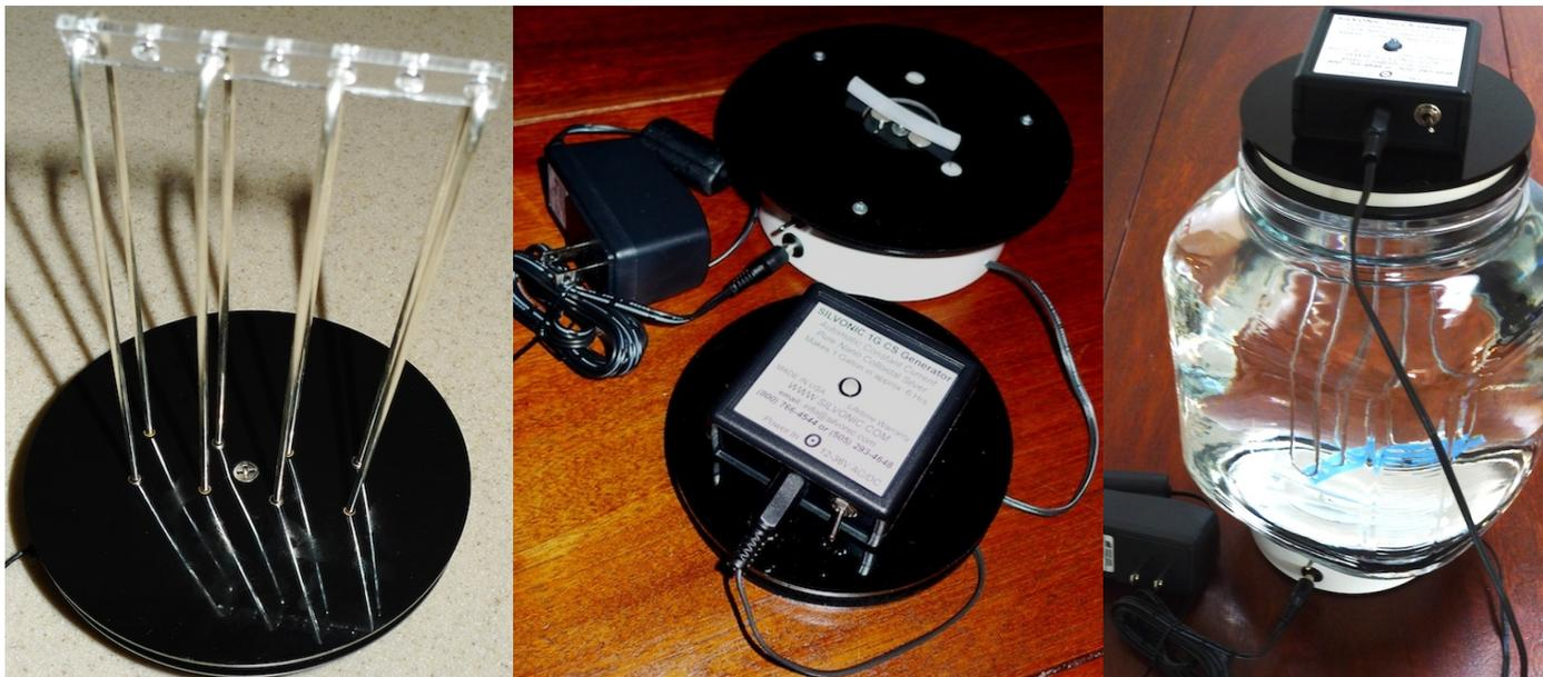
**Brewing time:** A one gallon batch should take about 6 hours to reach a conductivity reading of approximately 12  $\mu$ S. *Note:* Time varies with temperature... warmer water goes faster. Once a batch sits for a while and stabilizes, the reading will drop.
